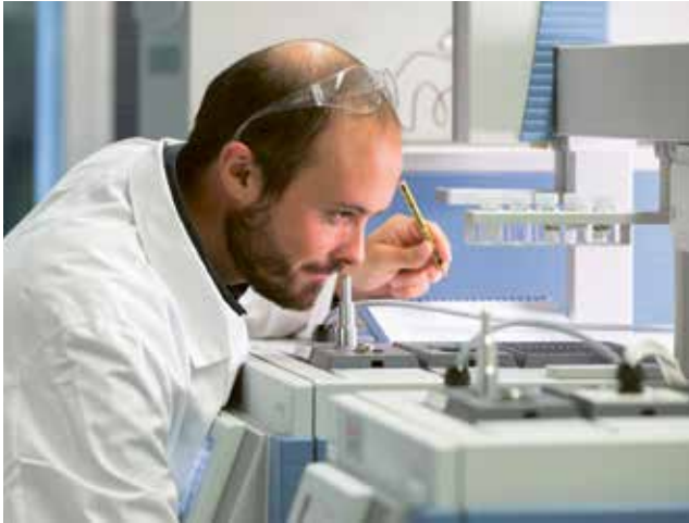
Lebensmittelextraktanalyse mittels Gaschromatographie-Olfaktometrie Food extract analysis by gas chromatography-olfactometry
