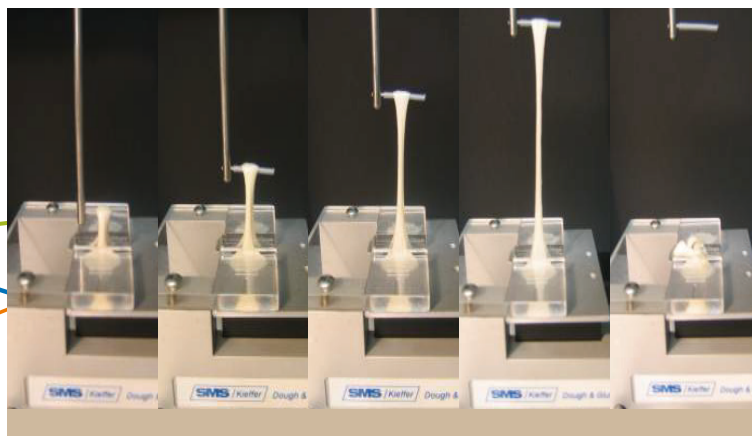
Tensile testing of dough for rheological analysis
